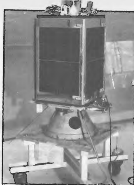
The amateur scientific satellite UOSAT, built at the University of Surrey, was launched by NASA on 6 October 1981. Its 515km-high polar orbit has a period of approximately 95 minutes. UOSAT's two main data beacons transmit on 145.825MHz and 435.025MHz; reception is possible during favourable passes on an ordinary amateur two-metre receiver with a quarter-wave whip aerial. A recorded news bulletin which also gives orbital predictions is available by telephone on Guildford (0483) 61202.
